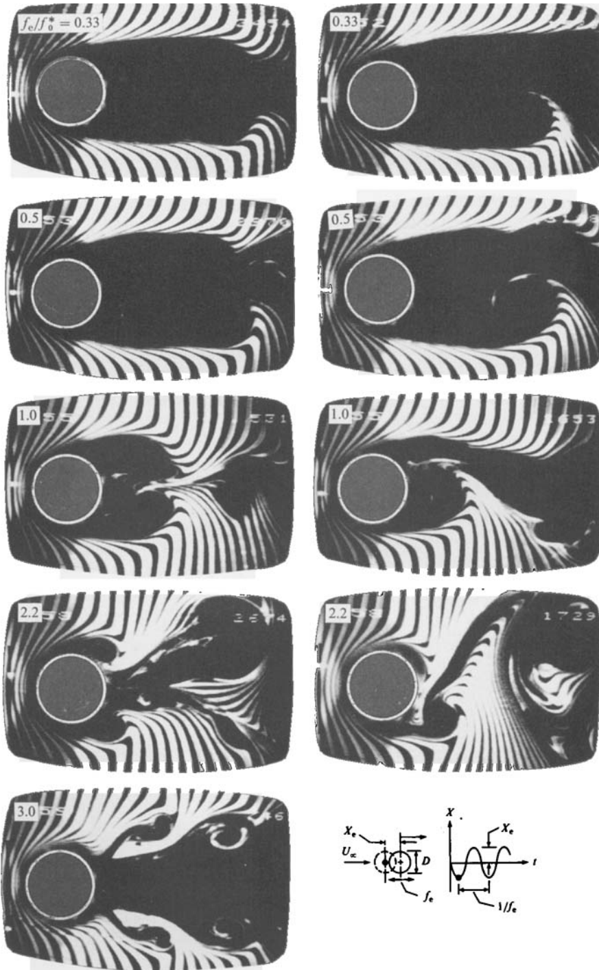
FIGURE 4. Comparison of symmetrical (left-hand column) and antisymmetrical (right-hand column) modes of non-synchronized vortex shedding from cylinder oscillating in streamwise direction as function of ratio of cylinder excitation frequency f_c^* from corresponding stationary cylinder. At f_c/f_0^* = 3 , vortex shedding is synchronized in symmetrical mode. All photos taken at instant corresponding to maximum upstream position of cylinder during oscillation cycle.
