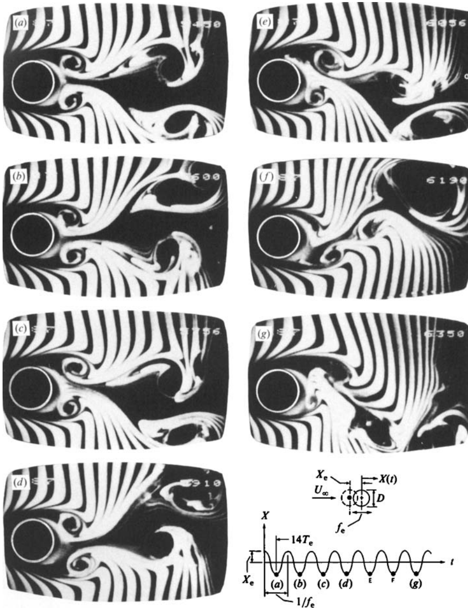
FIGURE 10. Ordered decay of symmetrical S mode of vortex shedding to antisymmetrical A mode for oscillations of cylinder in streamwise ( \alpha = 0^\circ ) direction. Cylinder was abruptly set into streamwise periodic motion at time fourteen cycles prior to upper left photo.
